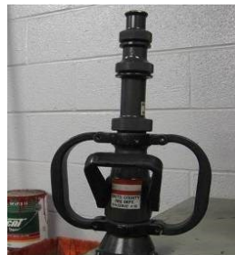
The nozzle pictured above is a 2 ½ smooth bore with stacked tips.
