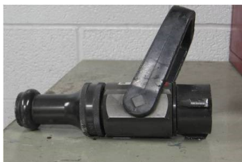
The nozzle pictured above is a 1 ¾ smooth bore. The tips most commonly carried on 1 ¾ nozzles are:
