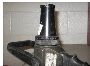
The nozzle pictured above is a 2 ½ smooth bore with stacked tips.
