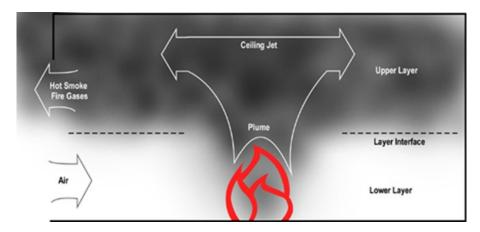
The interface where the hot gas layer and cool gas layer meet as the hot gases exit through an opening is referred to as the **neutral plane**. The series of pictures below shows the neutral plane up high in the opening to the fire compartment in the early stages of fire development. As the fire grows increased volume and pressure created in the fire compartment will push the superheated products of combustion and the neutral plane down lower within the compartment
