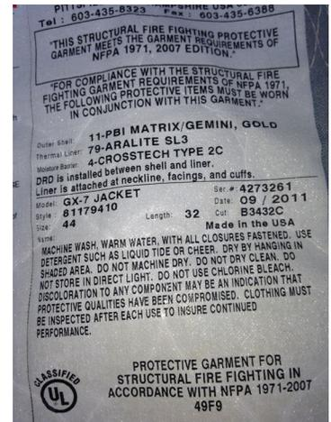
In each set of turnout gear manufactured there is a tag ensuring that the garment complies with the NFPA standard. It also lists the material that each protective layer is constructed of.
